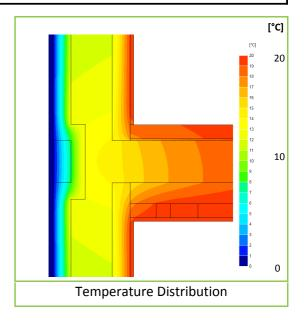
Party Floor with EPS insert 'thermal break', Standard Wall
